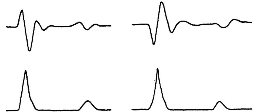
FIG. 1. Top: oscilloscope traces of  $dM/dt$  obtained with right and left circularly polarized light for a 3.1%  $\text{Eu}^{2+}$ -doped  $\text{CaF}_2$  crystal at 4.21°K. Bottom: monitor of the laser intensity.
