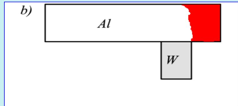
**Two possible mechanisms of metallization failure: (a) voiding and (b) surface erosion**
