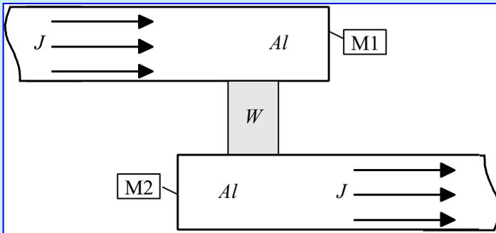
**Two-level metallization with the AL conducting lines interconnected by a tungsten via**
