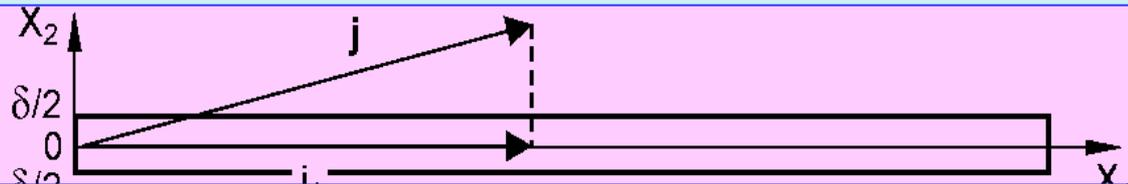
Frame of reference relative to a rectilinear grain boundary part.  $\delta$  is the grain boundary width,  $j_1$  is the projection of the current density vector on the  $X_1$  axis
