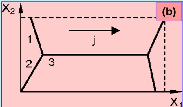
Conducting line (substrate and coating not depicted) (a); top view of the line segment under study (the digits denote rectilinear parts of the grain boundary converging in the triple point) (b)
